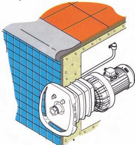
The pump can be connected either directly to the wall housing (compact assembly), or at a distance, except for the twin nozzle model which can only be installed remotely.
